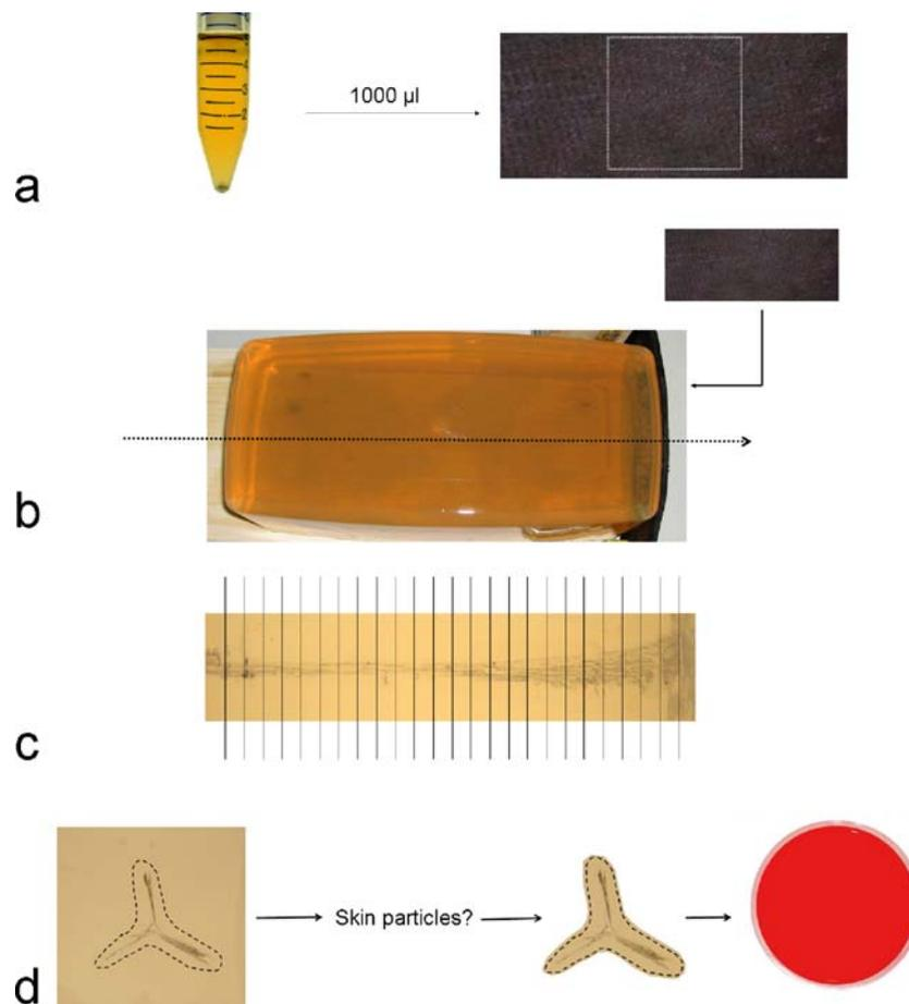
**Fig. 1** Schematic illustration of the experimental studies: **a** disinfected blue-coloured skin from a pig is wetted with a defined bacterial suspension; **b** shots are fired into the composite model of gelatin and skin from the gelatin side; **c** after firing the shot, the gelatin block is
