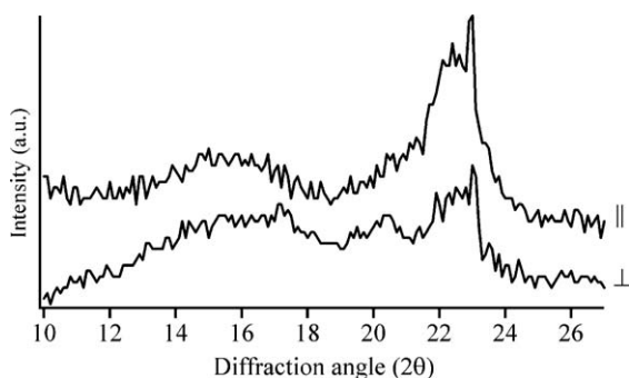
Fig. 4. WAXD spectra of sample N mounted in the parallel (top) and perpendicular (bottom) directions, in the angular range relative to cellulose.
